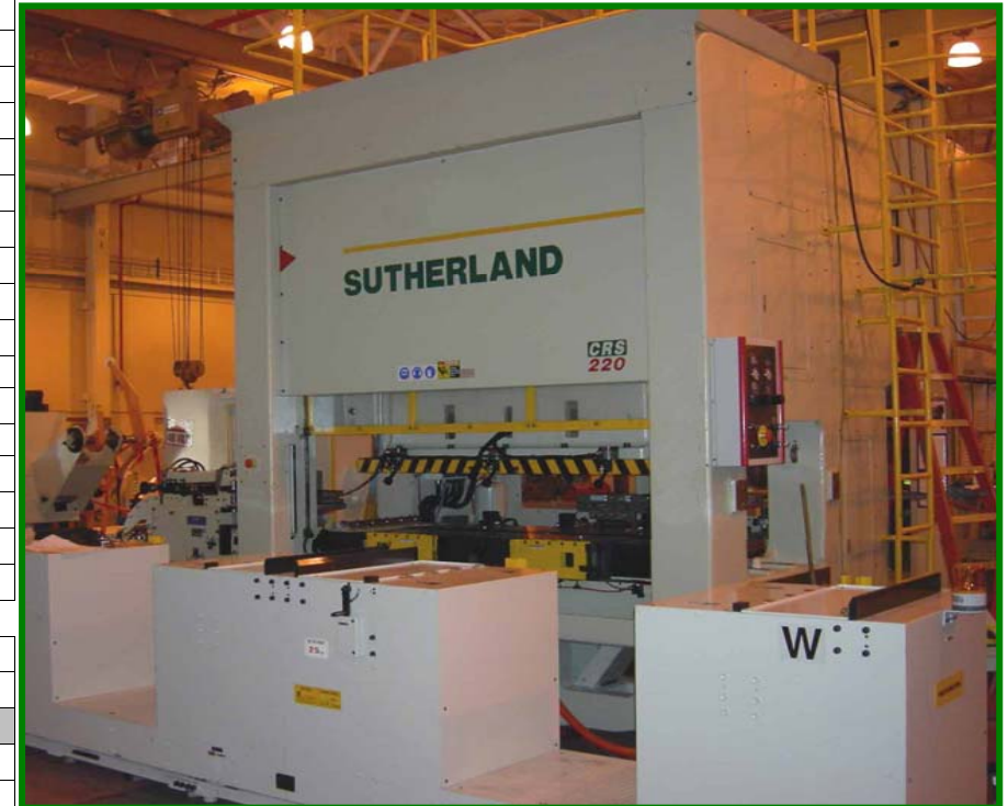
Ortlinghaus 406 Clutch & Brake, Ross air Valve, SMC Regulators, Wintriss-Sutherland Smart Pac II Press Control
