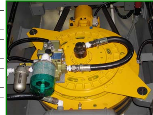
Ortlinghaus 406 Clutch & Brake, Ross air Valve, SMC Regulators, Wintriss-Sutherland Smart Pac II Press Control
