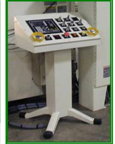
Ortlinghaus 406 Clutch & Brake, Ross air Valve, SMC Regulators, Wintriss-Sutherland Smart Pac II Press Control
